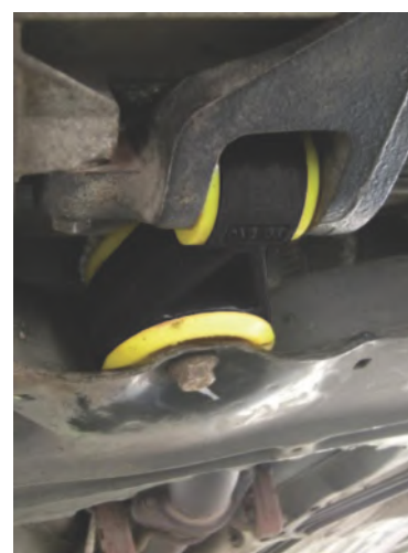
Figure 1 - fitted image of the polyurethane bush
