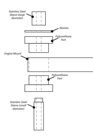
Figure 1 - diagram showing how all the parts fit together
