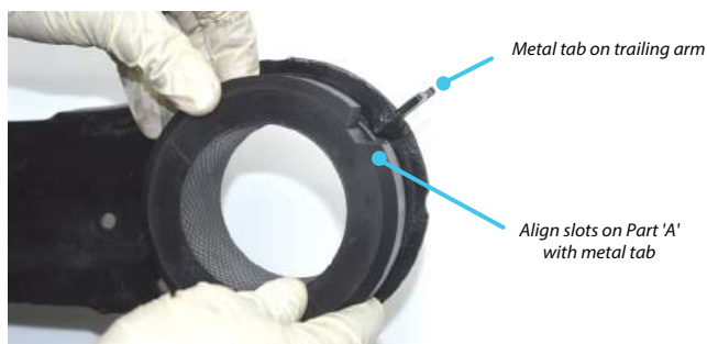
Figure 3 - Align slots on part A with welded tab on trailing arm
