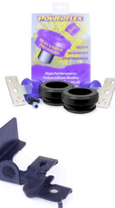
Figure 1 - Retain small metal bracket from original bush for refitting to new bush
