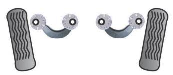
Sleeves adjusted to give maximum positive camber
