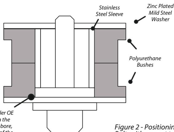
Figure 2 - Positioning of the Bolt, with respect to the other components
