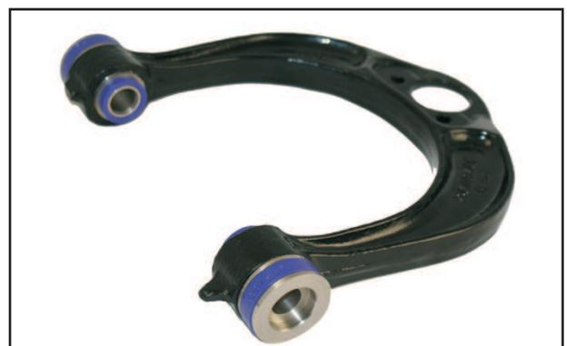
Photo 4. Cast arm showing complete bush assembly installed.
