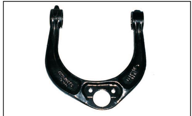
Photo 1. Cast arm with bushes removed.
