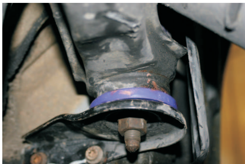
Fig 1. Rear beam mount - Assembled.
