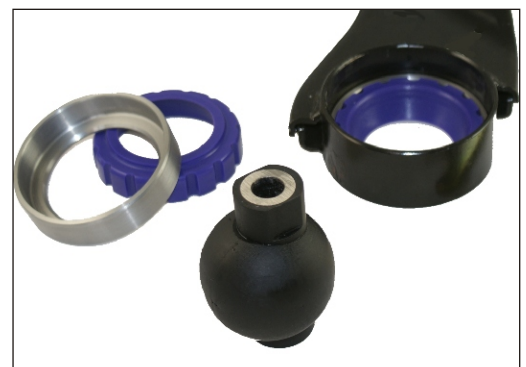
Fig 1. One shell and bush fitted to arm
