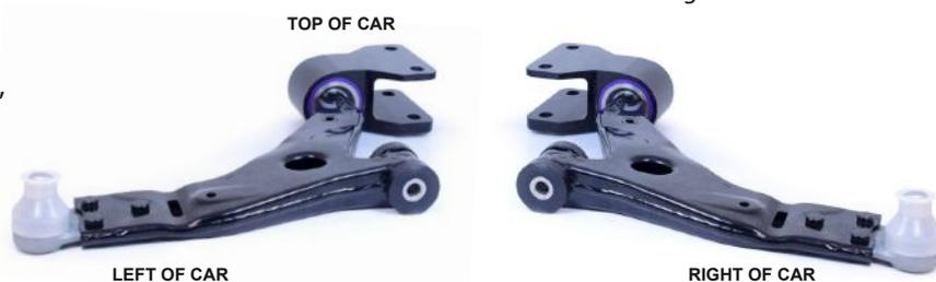
Figure 4 - Right-hand and left-hand bush and bracket assembly
