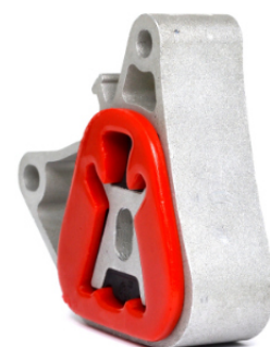
Figure 4 - showing polyurethane insert fitted inside the top engine mount
