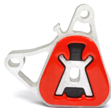
Figure 1 - showing polyurethane insert fitted inside the top engine mount
