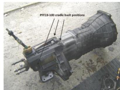
Figure 1- Location of OEM bushes to remove and replace.
