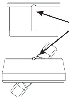
Align feature on shell with feature on shell for correct caster adjustment.
