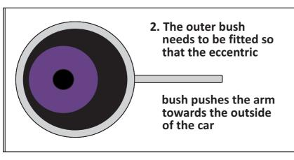
3. Please reset steering geometry after fitting any new suspension bushes
